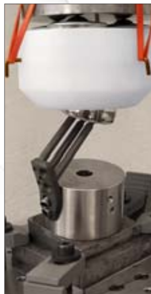
Set-up for biomechanical Targon® FN lab testing
